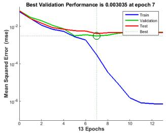
**Fig. 5:** Performance Graph: the graph of mean square error vs. epochs; blue line indicates the performance of trained data, green for validation data, red for test data. Best Validation Performance is 0.003035 at epoch 7.
