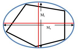
Fig. 3: The best fitting ellipse to a polygon with its major and minor axes; M<sub>i</sub> i.e. minor axis and M<sub>a</sub> i.e. major axis are shown by red lines
